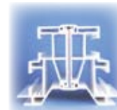
Multi-unit structural mull.
